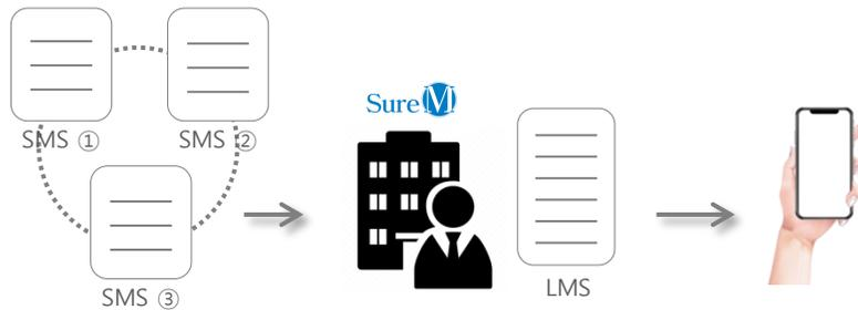
When overseas client send C-SMS, SureM combines SMS ①, ② and ③ into one long message(LMS) and end user can receive all the text as one message.
